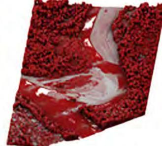
**Combined data with refraction correction, depth map and ground classification**
